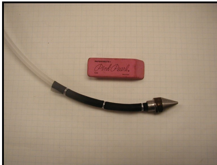
Fig. 6 - Well point, mesh screen, and sampling tube (Ref 7)
